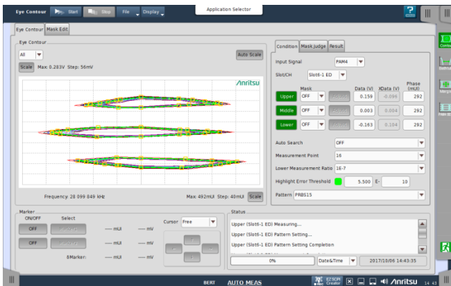
Example of Eye Contour Measurement at Input of PAM4 Signal
